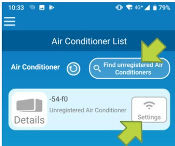
On the “Air Conditioner List” screen, tap the [Find unregistered Air Conditioners] button. The target air conditioner appears.
