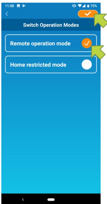
Tap [Remote operation mode] → Tap
