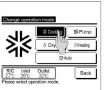
When the Change operation mode screen is displayed, tap the button of desired mode.
