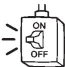
Unless the circuit breaker is installed, it could cause electric shocks.
