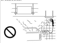
Locations with large amounts of oily smoke, such as food preparation areas. The unit will become inoperable if the filter or Heat Exchange Element become clogged with
