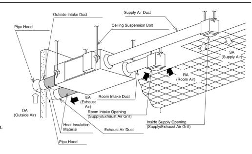
Note that when installing a unit body upside down, its printed indication is in a reversed position.
