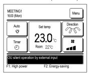
When "OU silent operation by external input" is displayed, the operation performed will be the same as the silent mode control (rapage 22) performed from the R/C.
