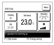
When you select to enable warming up by the Set ON timer by hour (FSF page 18) or Set ON timer by clock (FSF page 19), the operation will start 50 to 60 minutes earlier, which is predicted based on the previous warm up operation, so that the room will be close to the set temp by the time it reaches the operation start time. During the warm up operation, the message "In operation for warming up." will be displayed on the message display.
