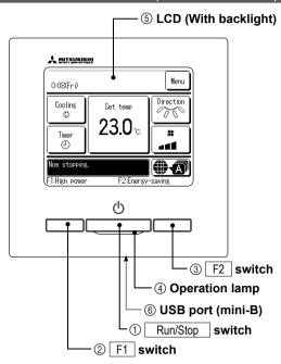
Touch panel system, which is operated by tapping the LCD screen with a finger, is employed for any operations other than the ① Run/Stop. ② F1 ③ F2 switches.
