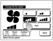
2 When the Change the fan speed screen is displayed, tap the button of desired fan speed.
