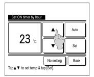
6 Select a desired temperature (at 1°C intervals) with the ▼ buttons. Or tap the Auto button and select the auto temp setting.
