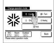
2 When the Change operation mode screen is displayed, tap the button of desired mode
