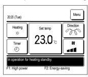
To prevent any cold air blowing out from the IO at the start of a heating operation, the unit stops the fan and displays "In operation for heating standby." on the message display.
