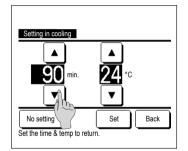
2 Set desired time and temperature with the buttons. When the Set button is tapped, contents of setting are confirmed, and the display returns to the last previous screen. When the No setting button is tapped. "-- min. -- °C" is displayed, and the "Automatic temp set back" is not performed.
