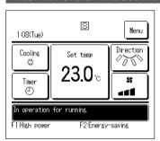
When one IU is controlled with 2 R/Cs, the following settings cannot be made on the sub R/C. It is necessary to use the main R/C. In case of the sub R/C, the icon  $\lceil S \rceil$  is displayed on the R/C screen.
