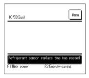
The refrigerant sensor is a component that requires regular maintenance
