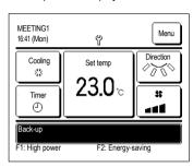
When the "Back-up" is displayed, contact dealer/company shown as the Contact company (rapage 24) immediately for checking.
