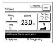
This does not indicate a failure; the message indicates that the unit is controlled through a central control device.
