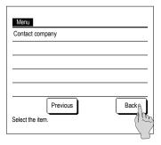
**3** When the Back button is tapped, the display returns to the TOP screen.
