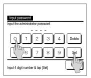
When an item is referenced to Administrator password it this manual, the Input password screen is displayed after selecting the menu.
