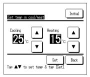
3 Use the ▲ ▼ button to set the temperature, and tap the Set button. Temporarily determine the set temperature. The allowable range is as follows:
