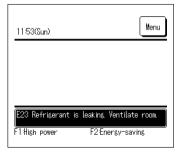
This message is displayed if the refrigerant sensor detects a refrigerant leak.
