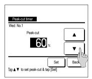
9 Set the peak-cut %. Set the peak-cut % with the buttons. The peak-cut % can be set at 0%, 40%, 60% or 80%. The lower the peak-cut % is, the higher the effect
