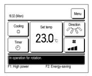
When rotation, capacity back-up, or fault back-up operation is enabled during installation, a message indicating the operation that is set and running will be displayed on the message display.
