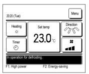
When frost forms on the OU, the heating performance will decrease. This will cause the unit to automatically switch to defrost operation, and hot air will stop blowing out from the IO.
