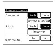
2 Select Enable/Disable for Power control. When you select Enable, the set temperature is gradually adjusted to ±3.0 based on the amount of activities.
