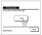
3 Acknowledge screen for the Filter sign reset screen is displayed.
