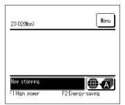
When the operation stops, all operation buttons on the screen turn off. When the set lighting time of backlight (Es page 16) is counted up, the backlight turns off.
