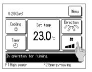
1 Tap the Change the fan speed button on the TOP screen.
