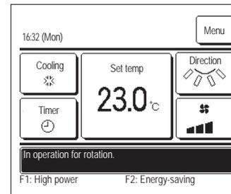
When rotation, capacity back-up, or fault back-up operation is enabled during installation, a message indicating the operation that is set and running will be displayed on the message display. Refer to the installation manual on how to make these settings.
