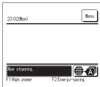
When the operation stops, all operation buttons on the screen turn off. When the set lighting time of backlight (see page 16) is counted up, the backlight turns off.
