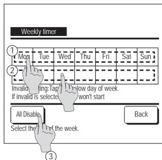
3 When a desired day of the week ① is tapped on the display, contents of current setting for the day are displayed. (P.5)
