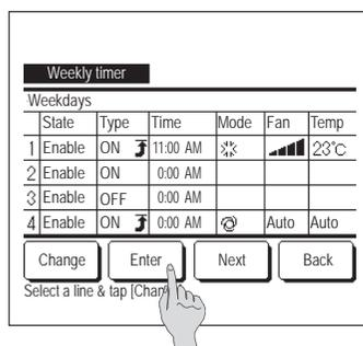
12 Display the setting contents check screen. To register the setting, tap the **Enter** button.
