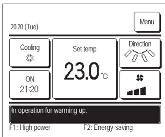
When you select to enable warming up by the Set ON timer by hour (☞page 18) or Set ON timer by clock (☞page 19), the operation will start 50 to 60 minutes earlier, which is predicted based on the previous warm up operation, so that the room will be close to the set temp by the time it reaches the operation start time. During the warm up operation, the message “In operation for warming up.” will be displayed on the message display. This message will disappear at the time set for operation start.
