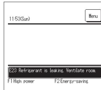
This message is displayed if the refrigerant sensor detects a refrigerant leak.
