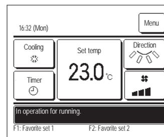
1 When you press the **F1** (**F2**) switch, the operation mode, set temp, fan speed, flap direction registered to Favorite set 1 or Favorite set 2 will be enabled.
