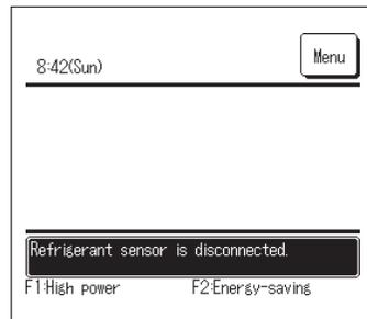
This message is displayed if the refrigerant sensor is disconnected.
