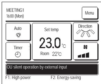
When “OU silent operation by external input” is displayed, the operation performed will be the same as the silent mode control (☞page 22) performed from the R/C.
