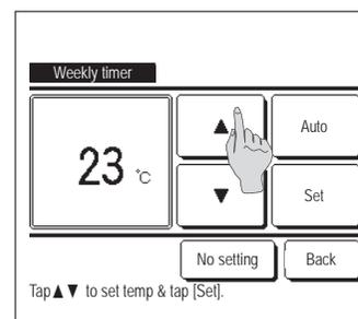
9 Select a desired temperature (at 1°C intervals) with the ▲▼ buttons. Or tap the [Auto] button to select the Auto temp setting.
