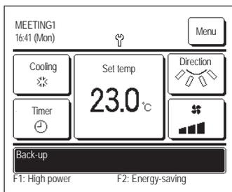
When the “Back-up” is displayed, contact dealer/company shown as the Contact company (☞page 24) immediately for checking.
