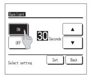
1. When tapping [Backlight] on the [Initial settings] menu screen, the [Backlight] setting screen is displayed.
