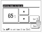
**4.** On the setting screen of each item, if the Set button is placed, the setting content can be confirmed by tapping Set button.
