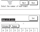
3. Set the name of HP unit to be added to the HP unit No. button.
