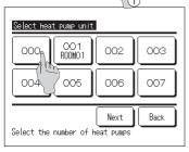
5. The selection screen of heat pump unit is displayed.
