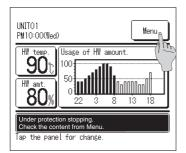
**1.** The message of [Under protection stopping] is displayed at the message display section.
