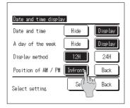
**1.** When tapping [Date and time display] on the [Initial settings] menu screen, the [Date and time display] screen is displayed.
