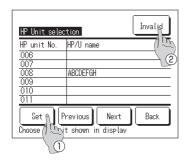
**1.** When tapping the [HP unit selection] on the [Administrator settings] menu screen, the [HP unit selection] screen is displayed.
