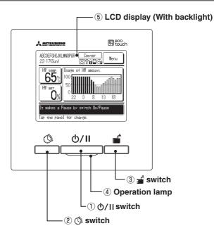
Touch panel system, which is operated by tapping the LCD screen with a finger, is employed for any operations other than the ①Run/Pause, ②Schedule setting and ③Operation to fill up switches.
