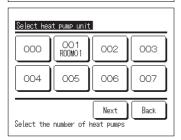
If the multiple heat pump units is connected to the remote control, the list of heat pump units (Address No.) is displayed.
