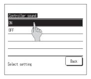
1. When tapping [controller sound] on the [Initial settings] menu screen, the [Controller sound] setting screen is displayed.
