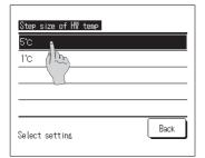
**1.** When tapping the [Step size of HW temp] on the [Administrator settings menu screen, the [Step size of HW temp] menu screen is displayed.
