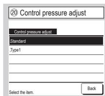
Set the control pressure when connecting the outdoor air conditioning unit to the Multi (KX) System.
