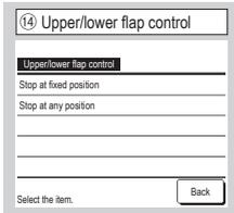
Stop at fixed position The upper/lower flap can be set to stop at one of four positions.
