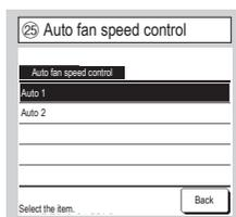
Set the switching range of the fan tap at the auto fan speed setting.
