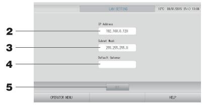
2. Setting and viewing the IP Address (Factory default: 192.168.0.120)
