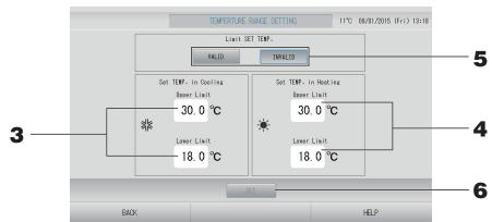
**3.** Press Upper/Lower limit (°C) of SET TEMP. in Cooling. Select temperature by pressing or button and OK button.
