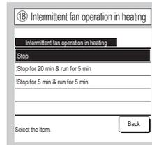
Select the fan control after the residual fan operation following stop and thermo-OFF in heating mode.
