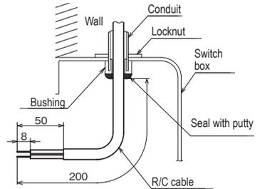
② When wires are passed through the bottom case, fix the bottom case at 2 places on the switch box.
