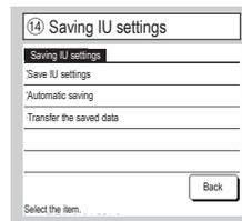
**Save IU settings** All settings of the IUs connected to the R/C are saved in the R/C.
