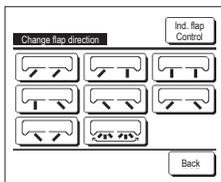
4 Tap the desired flap direction. After selecting the flap direction, the display returns to the Select flap screen. (**≡P 1**)
