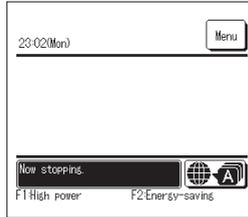
When the operation stops, all operation buttons on the screen turn off. When the set lighting time of backlight is counted up, the backlight turns off.
