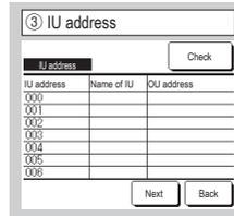
When 8 or more units are connected, further data are displayed on the next page. When the  button is tapped after selecting an IU address, the fan of the selected IU can be operated. ⇒ ④
