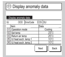
The operation data obtained just before the occurrence of an error are displayed.
