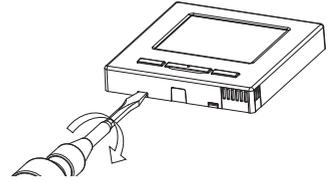
To disassemble the R/C case into the upper and lower pieces after assembling them once
