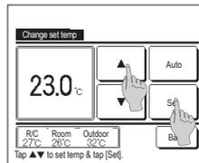
2 When the Change set temp screen is displayed, select the temperature as desired with using **▲** **▼** buttons.
