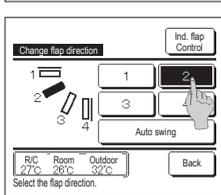
2 When the Change flap direction screen is displayed, tap the button of desired flap direction.
