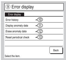
Date and time when error occurred, IU address and Error Code are displayed.
