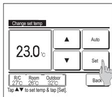
4 When the **Set** button is displayed on the setting screen for each item, tapping this button confirms the setting.
