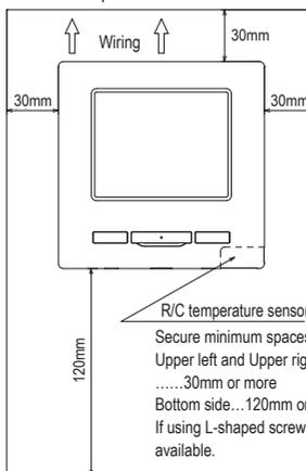
Secure minimum spaces for disassembling the case.
