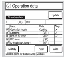
After read the indoor unit data, the operation data at the time of reading are displayed. Tapping the  button to update the data. To automatically update data and display, up to six items can be selected. Tapping the  button after selecting six items changes the display to ⑧ .
