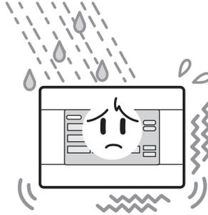
If it is installed in an area exposed to humidity, splashing water or high vibration, it will cause malfunctions.
