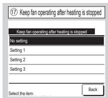
Select the residual fan operation time period after stopping and the thermo-OFF in heating mode.
