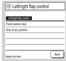
Fixed position stop The left/right flap can be set to stop in eight different patterns.
