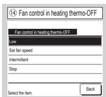
Set the fan speed at the heating thermo-OFF.
