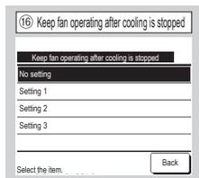
Select the residual fan operation time period after stopping and the thermo-OFF in cooling mode.
