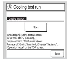
This can be operated while cooling is stopped. When the room temperature is too low to start the cooling test run, it operates for 30 minutes by decreasing the set temperature to 5°C.
