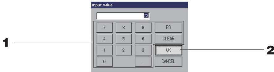
**1. Press the button of the numerical value to input.**
