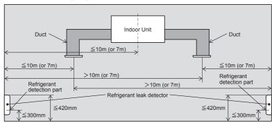
Indoor Unit and Each Inlet/Outlet are over 10m (or 7m) without Ceiling (Side view)
