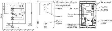
To disassemble the refrigerant leak detector case into the upper and lower pieces after assembling them once
