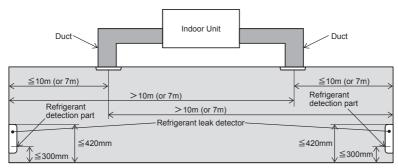
Each Inlet/Outlet are over 10m (or 7m) with Ceiling (Side view)
