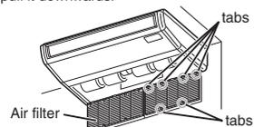
When attaching the filter, insert the filter into the tabs of the inlet grille.
