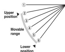
Note : If the upper limit position number and the lower limit position number are set to the same position, the louver is fixed at that position. And auto swing does not function.
