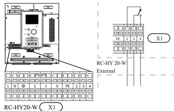
If the relay is to be used for control voltage, bridge the supply from terminal block X1:1 to X1:2 and connect neutral and control voltage from the external additional heat to X1:0 (N) and X1:4 (L).
