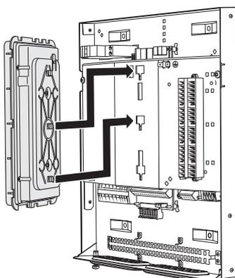
3. Align the two lower mountings on the reverse of the display unit with the two upper holes in the panel as illustrated.
