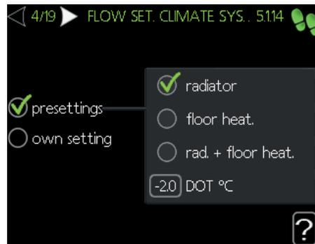
The type of heating distribution system the heating medium pump works towards is set here.
