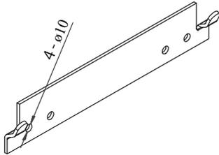
2. Insert HSB60-W in the bracket mounted to the wall.
