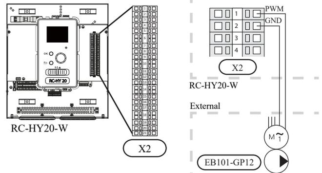
**Connection between controller and 3-way valve (QN10/QN12)**
