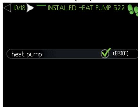
Enable heat pump (EB101) here.
