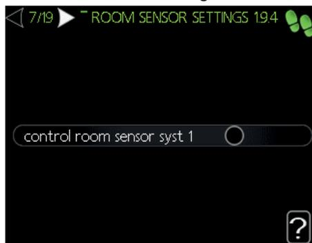
Activate and set the room temperature sensor RTS40M (if connected) for each climate system
