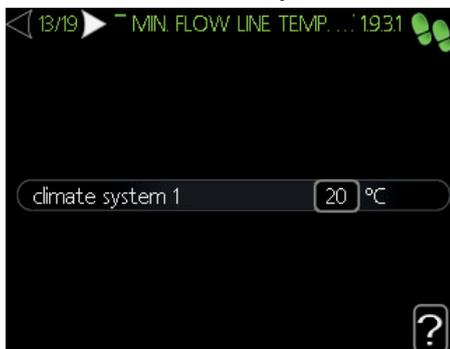
Set the minimum flow line temperature of the climate system.
