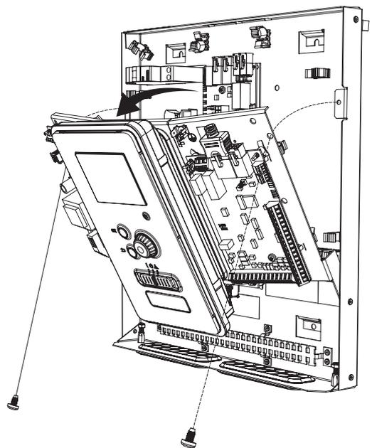
The display may need to be moved for easier access when connecting electrics. This is easily done by following these steps.
