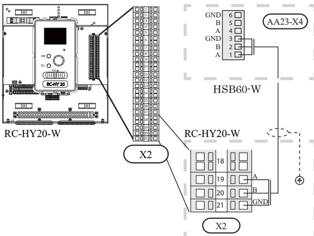
**Connection between controller and circulation pump (GP12)**
