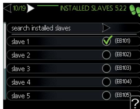
Search for installed slaves and enable them (if connected) here. If everything is correct the units are automatically selected after searching for installed slaves.
