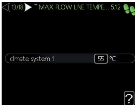
Set the maximum flow line temperature of the climate system.
