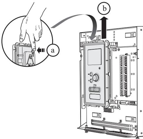
1. Press in the catch on the upper rear side of the display unit towards you (a) and move the display unit upwards (b) so that the mountings unhook from the panel.
