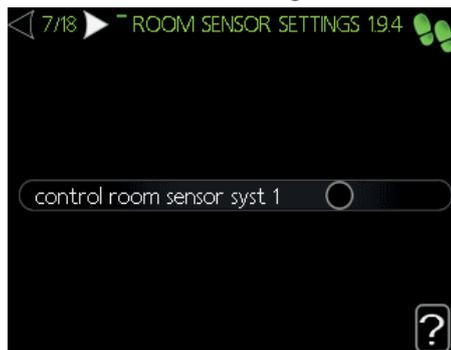
Activate and set the room temperature sensor RTS40M (if connected)
