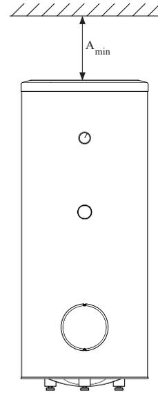
$A_{min}$  is required on top to replace anode bar, and 500 mm is required in front to replace immersion heater if equipped.
