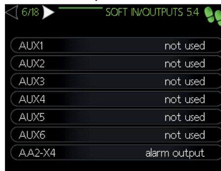
Set the function of each input and output for each terminal (if connected)
