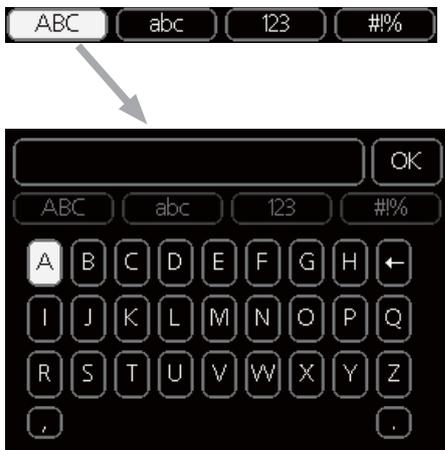
Depending on the menu, you can gain access to different character sets which you can select using the control knob. To change character table, press the Back button. If a menu only has one character set, the keyboard is displayed directly.
