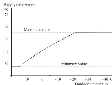
The figure at the end of the curve indicates the curve number. The figure beside the thermometer icon gives the curve offset. Use the control knob to set a new value.
