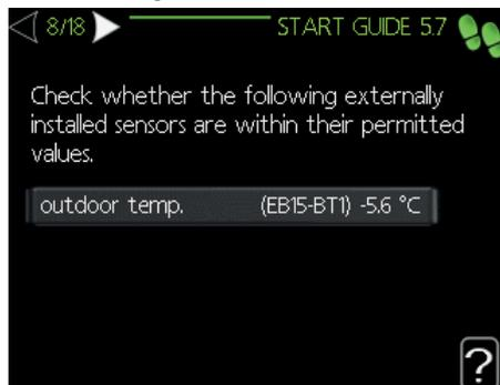
Check if the values of the shown temperature sensors are correct.
