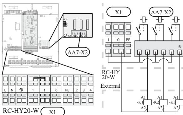
If the relays are to be used for control voltage, bridge the supply from terminal block X1:1 to X2:1, X2:3 and X2:5 on additional relay board (AA7). Connect the neutral from the external additional heat to terminal block X1:0.
