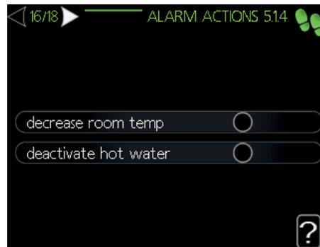
Set how to control the heat pump in case of alarm.
