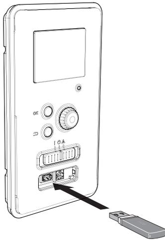
RC-HY20/40-W is equipped with a USB socket in the display unit. This USB socket can be used to connect a USB memory to update the software, save logged information and handle the settings in RC-HY20/40-W.
