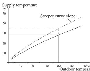
The optimum slope depends on the climate conditions in your location, the type of heating device (radiators or under floor heating) and how well insulated the house is.
