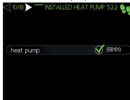
Enable heat pump (EB101) here.
