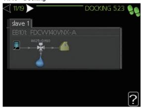
From factory docking comes pre-set as shown above – heating and hot water only. If necessary, docking needs to adjust manually according to installation type.
