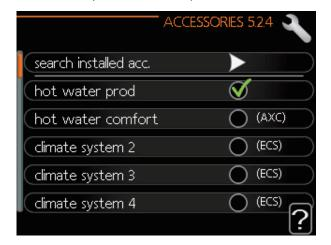
Set which accessories are installed on the installation here.
