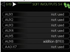
Set the function of each input and output for each terminal (if connected).
