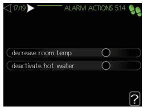
Set how to control the heat pump system in case of alarm.
