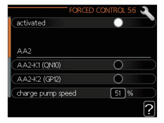
You can force control the different components in the controller and any connected accessories here.
