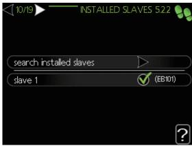
Search for installed slave and enable it (if connected) here. If everything is correct, the unit is automatically selected after searching for installed slaves.
