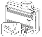
Check that the reception buzzer sound "pip" is emitted from the indoor unit.
