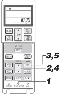
Press the TIME SET UP switch.
