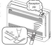
Check that the reception buzzer sound "pip" is emitted from the indoor unit.
