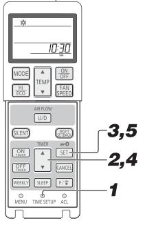
Press the TIME SET UP switch.
